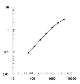
the concentration on the x-axis and draw a best fit curve through the points on the graph. This procedure will produce an adequate but less precise fit of the data. If samples have been diluted, the concentration read from the standard curve must be multiplied by the dilution factor.
